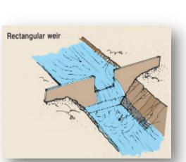
designed perpendicular to the flow direction in the stream beds to decrease the velocity of water and to keep some amount of water behind them. This causes a decrease in the volume of flowing water and that is helpful in sudden flood events. They have generally an open part on the top which lets water to flow when it reaches a certain level. Permitting flow rate is defined by the dimensions and the shape of the opening. Typical types of openings are trapezoidal, rectangular, and triangular.
