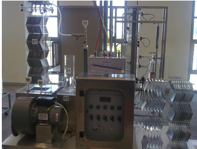
Figure 1. Cooling Tower Apparatus
