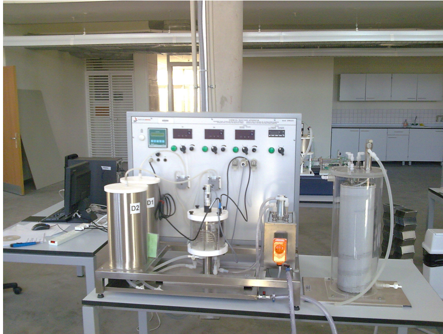
Figure 1. Chemical Reactor Apparatus
