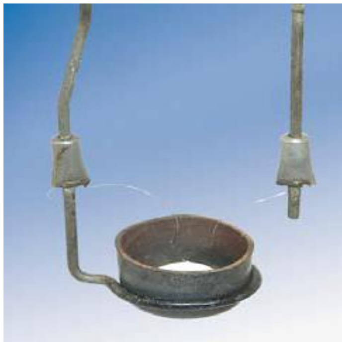
Figure 3. Closer view of sample capsule and ignition wire.
