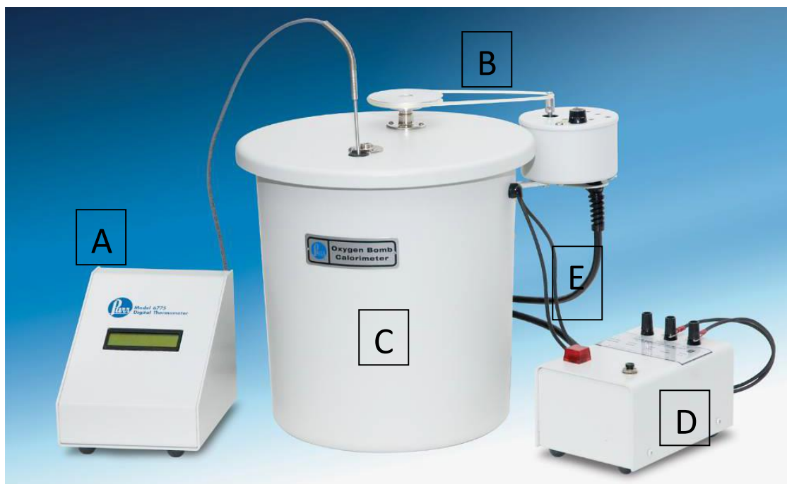
Figure 1. Overview of the Oxygen Bomb Calorimeter. A: Temperature display connected to thermocouple, B: stirrer shaft, C: Calorimeter Cover, D: Ignition Unit, E: cables entering the bomb for ignition.
